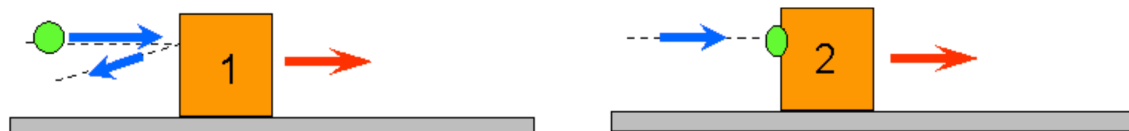
Figure 3. (Unit 11) Two balls of equal mass are thrown horizontally with the same initial velocity. They hit identical stationary boxes resting on a frictionless horizontal surface. The ball hitting box 1 bounces back, while the ball hitting box 2 gets stuck. Which box ends up moving faster?
