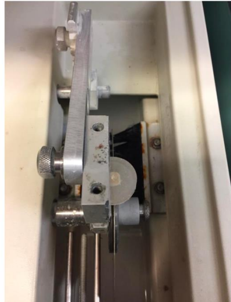
Figures 14, and 15: IsoMet 1000 saw (Buehler, Lake Bluff, IL, USA) used to split samples.
