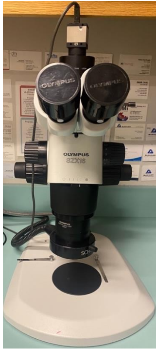
Figure 20: Olympus SZX 16 (Olympus, Tokyo, Japan) stereomicroscope with a digital camera (Ueye 3.90, Obersulm, district of Heilbronn, Germany).
