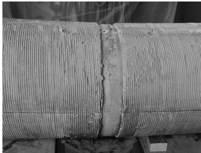
Fig. 23. Damage in the concrete core at the splice location
