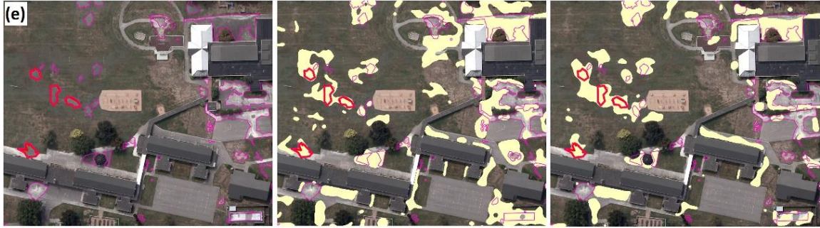
Figure 3-16. Binary classification results of Model 1 (RGB-based model in the middle column) Model 6 (preferred model in the right column) with Sanon et al. (2023) liquefaction polygons (in thick red) and validation labels (in magenta) overlaying the model prediction (in yellow).
