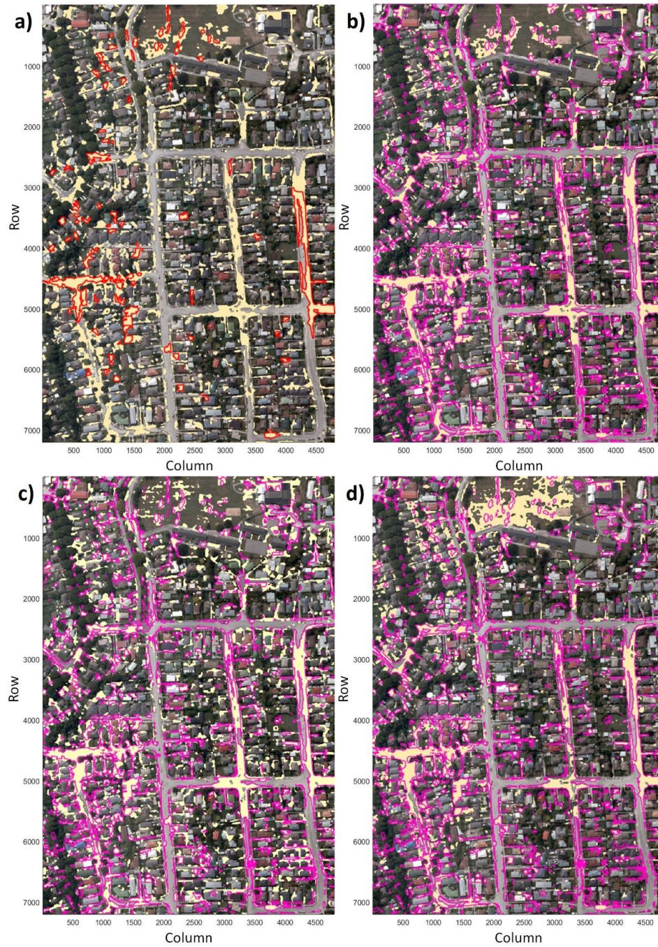
Figure 3-15. a) Binary classification results of Model 6 (preferred model) with Sanon et al. (2023) liquefaction polygons (in red) overlaying the model prediction (in yellow); b) Model 6 output (in yellow) compared with validation labels (in magenta); c) Supervised classification output with validation labels overlaid; d) Model 1 (RGB-based model) classification output with validation labels overlaid.
