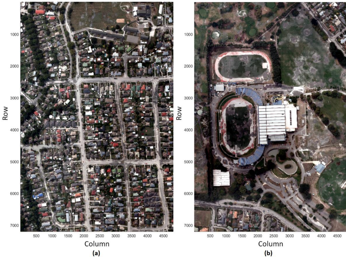
Figure 3-2. a) The image tile used for model development and evaluation. b) The image tile used for further model application. Both tiles have a resolution of 10 centimeters, and each tile is 720-by-480 meters in size. Linear stretching is performed on the image for better visualization contrast.
