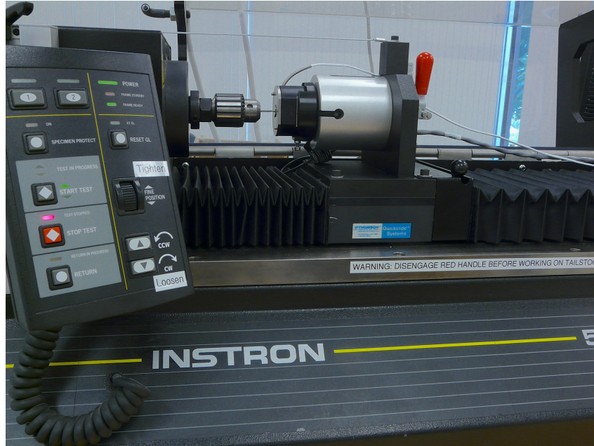
Figure 16: The Instron 55MT torsion test machine, ready for a test
