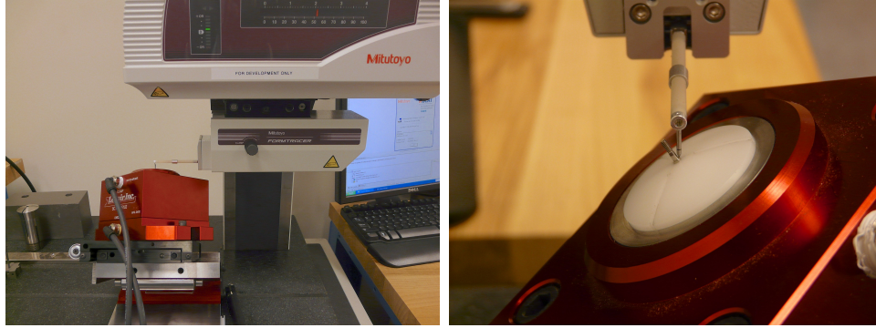
(a) Profilometer, as used to measure the roughness of the flat screws (b) Close-up of profilometer and fixturing, showing stylus tracing the screw seating surface
