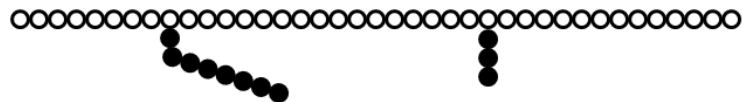
Figure 1.2 Different types of polymer chains. Black and white circles indicate different type of monomers.
