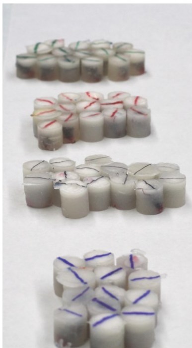
Figure 2: Samples embedded into orthodontic resin (Dentsply Caulk)
