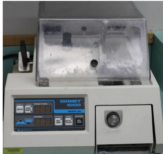
Figure 3: Low speed sectioning wheel isomet 1000 (Buehler, Germany)
