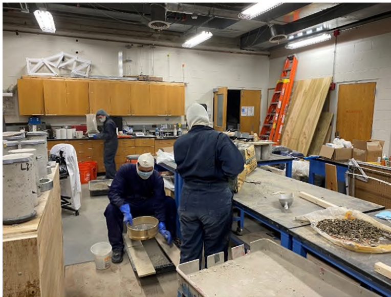
Figure 151 The preparation of materials (sieving aggregates) for casting at Tufts University (March 2023).
