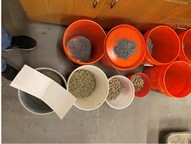
Figure 152 Types of aggregates used in the casting of new concrete cylinders.
