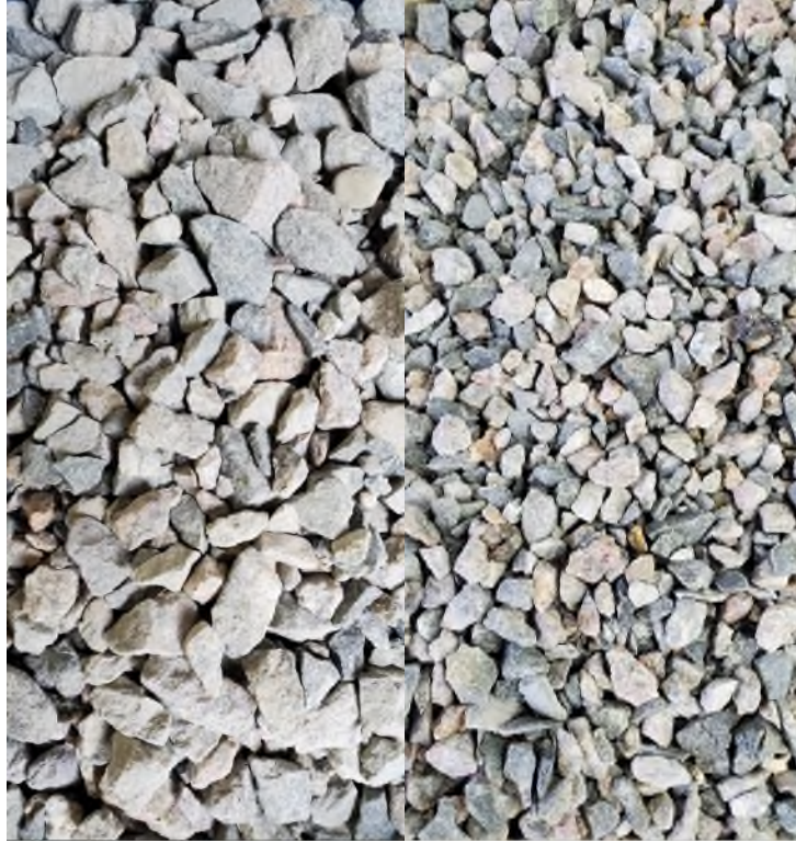
Figure 160 Coarse crushed granite aggregate; Left) max aggregate size of \frac{3}{4} in; Right) max aggregate size of \frac{3}{8} in.
