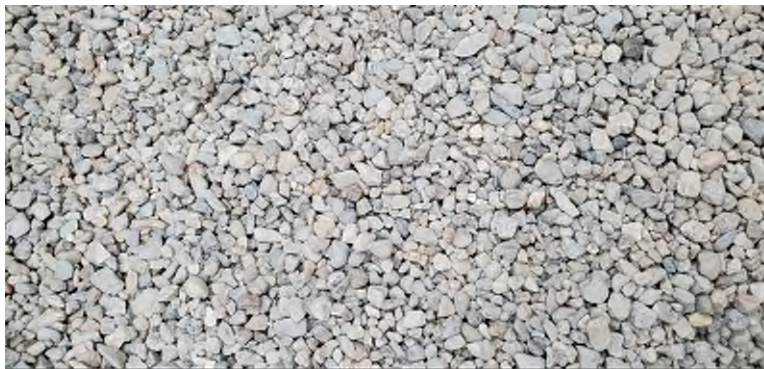
Figure 161 River based round aggregate with max size of \frac{3}{8} in.
