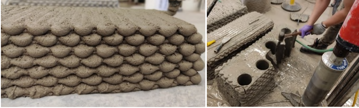
Figure 132 3D-printed beam (left) and the coring procedure for production of cylindrical specimens (right).
