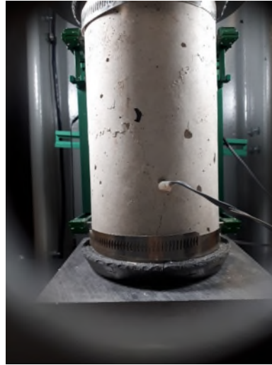
e) N=11,300, few hundreds of cycles before failure
