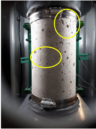
a) N=14,400 first visual cracks
