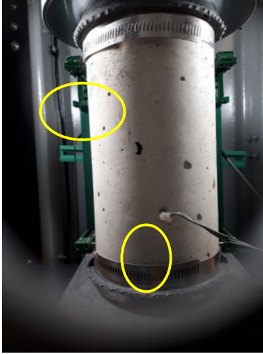
a) N=7,300 first visual cracks
