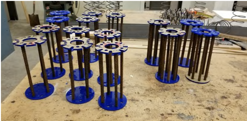
(c) Reinforced concrete specimens before casting
