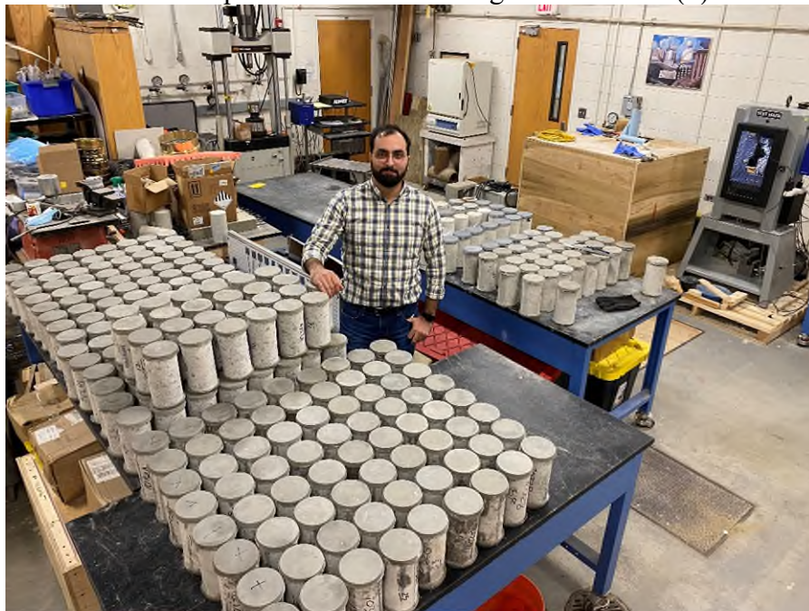
(e) Final cast concrete samples with different aggregate sizes
