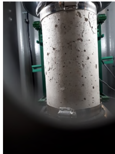
e) N=23,500, a few hundreds cycles before failure
