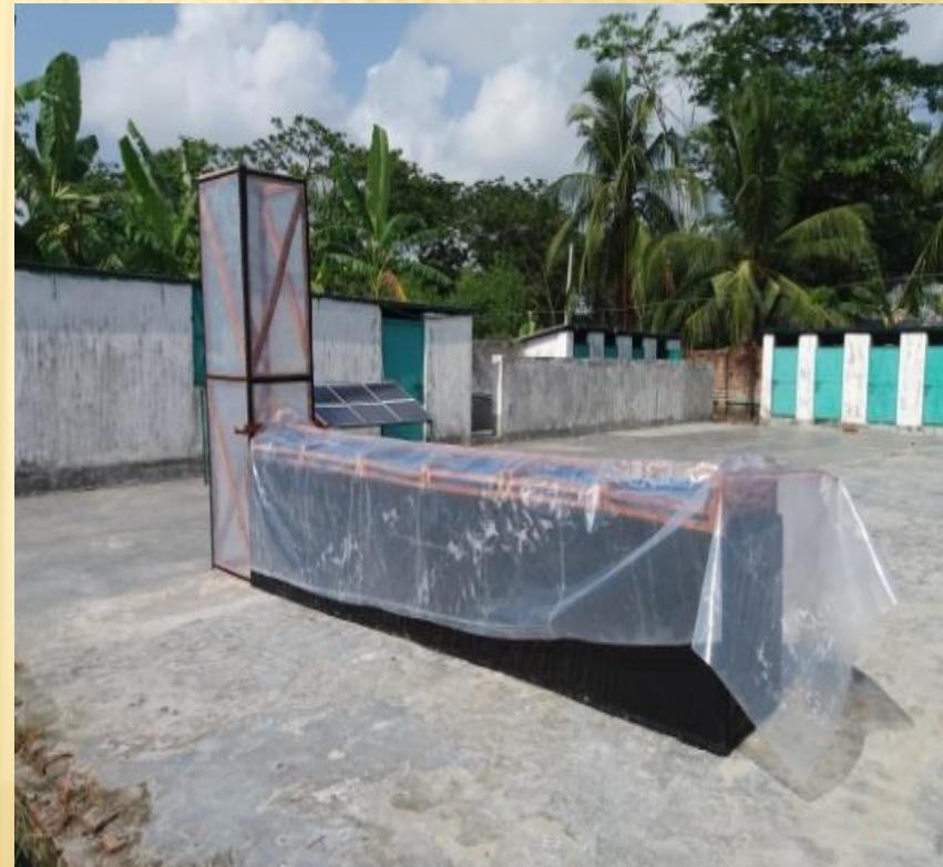
Figure 3: UC Davis chimney solar dryer
