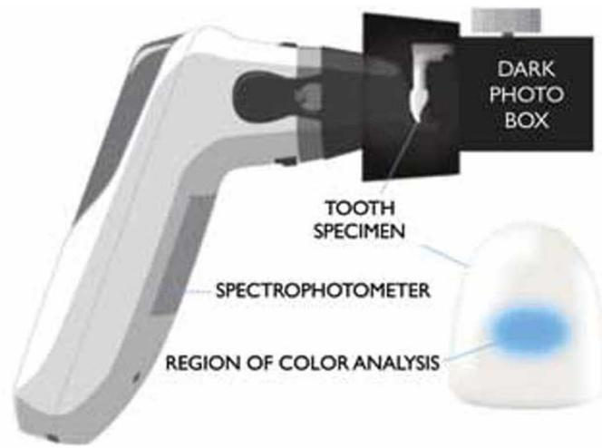
Figure 2 SpectroShade Micro (MHT, Italy).
