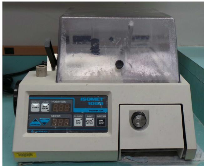
Figure 3 IsoMet 1000 (Sectioning Machine)
