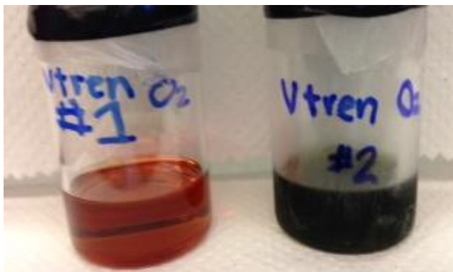
Figure 3A.16. Left: Toluene solution of V[(Me_3SiNCH_2CH_2)_3N] (1 mM) after addition of pure O_2 at ambient temperature. Right: Toluene solution of V[(Me_3SiNCH_2CH_2)_3N] (1 mM) after addition of pure O_2 at low temperature ( \approx -78\text{ }^\circ\text{C} ). 100% O_2 (extra dry grade) was sparged directly into each vial for approximately 15 s.
