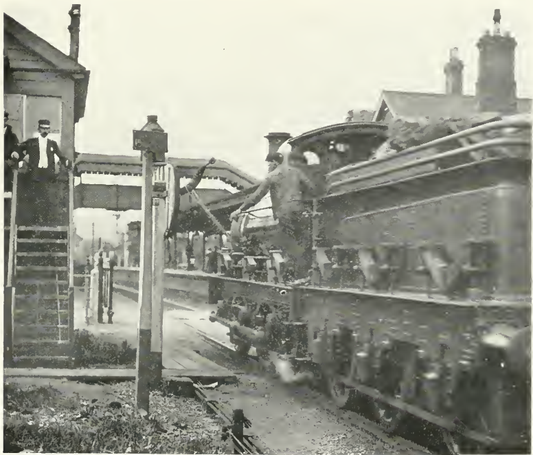
APPARATUS FOR SINGLE LINE WORKING. ENGINE-DRIVER DROPPING "STAFF" AT SPEED, G. W. R.
