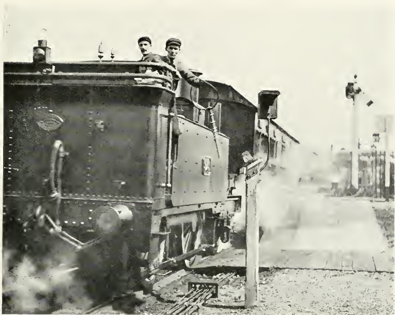
APPARATUS FOR SINGLE LINE WORKING. ENGINE-DRIVER PICKING UP "STAFF" AT SPEED, G. W. R.
