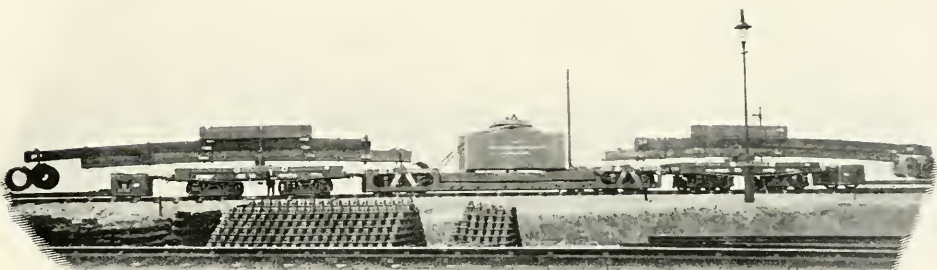
90-TON CASTING LOADED ON G C. R. WAGONS, SUPPORTED BY CANTILEVER ARRANGEMENTS.
