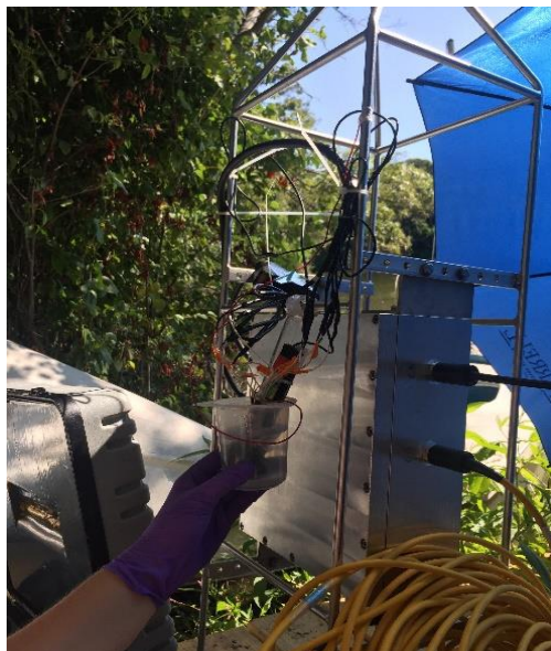
Figure 17 . The experimental setup including the modified potentiometer in a waterproof aluminum chassis and array of electrodes during field calibrations
