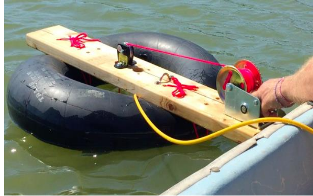
Figure 18 . The inner tube and pulley system that supported the cage, electronics and electrodes during in-situ measurements
