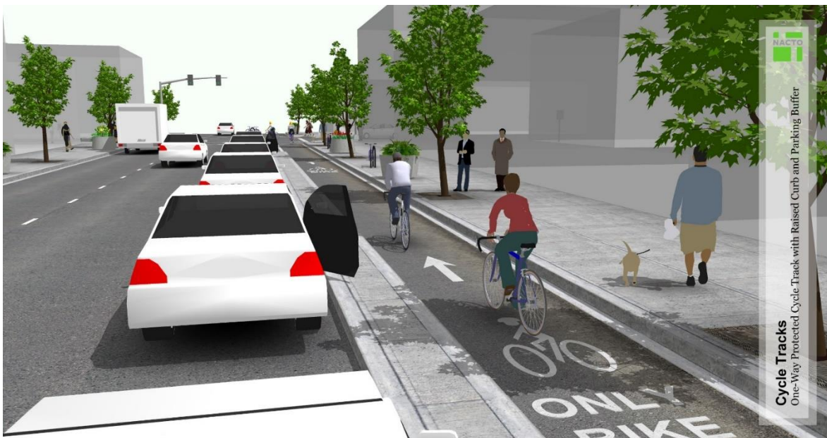
Figure 2: Cycletrack Protected by Curb (NACTO 2014)
