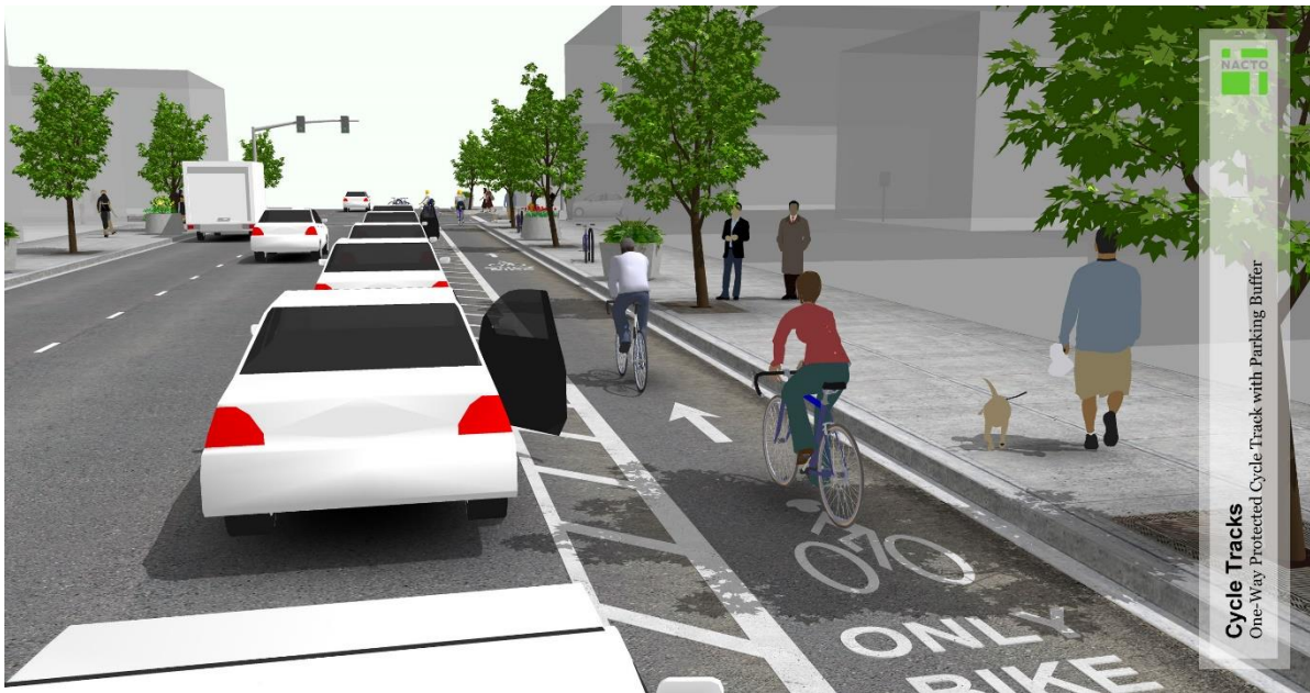
Figure 3: Cycletrack and Buffered Lane (NACTO 2014)
