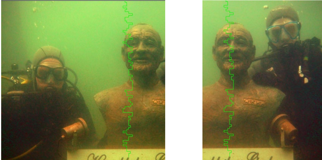
Fig. 4.3.5: Generation of seam line using Alpha-winzorized correlation
