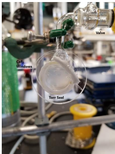
Figure 2.2 – A typical glass cell with \text{CaF}_2 windows attached by Torr Seal Epoxy.
