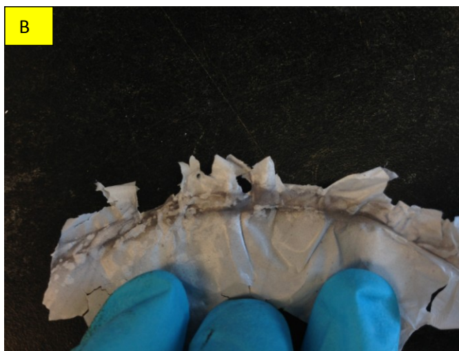
Figure 18: A) Stationary circular collector used initially for spinning scaffolds. B) For the samples prepared using this collector, uneven distribution of \text{Fe}_3\text{O}_4 was noticed.
