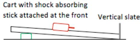
*Figure 3.* Vertical slate on the track and shock absorbing stick on the cart.
