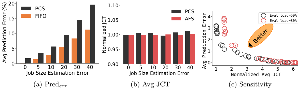
Figure 3.10: Shows the effects of error in job size and load estimation. a) compares the average Pred_{err} using PCS and FIFO [193] with varying job size estimation error. b) compares the avg JCT of PCS and AFS [106] under the same error. c) shows sensitivity of WFQ configs to load changes.
