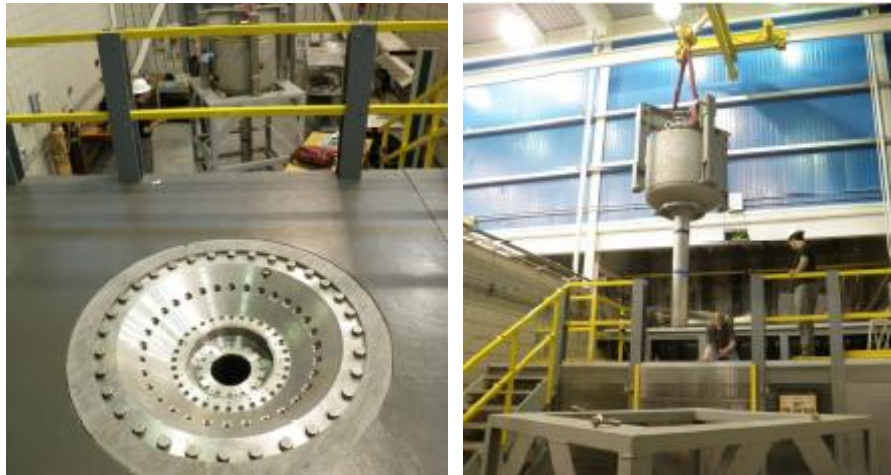
Figure 6.12 – Cryostat (right) being lowered into the magnet bore shown on the left.
