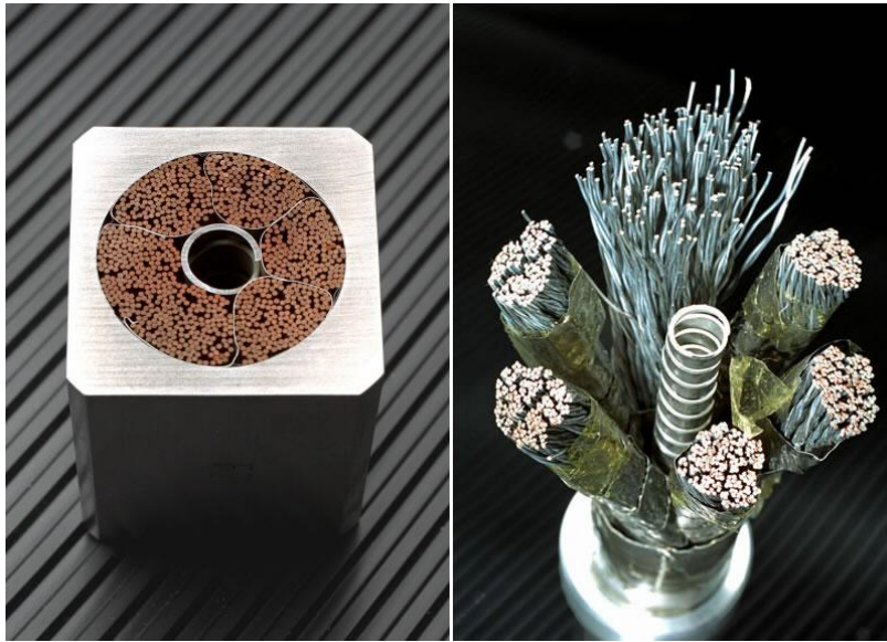
Figure 1.3 – Cable-in-Conduit Conductors (CICC) for ITER magnets [11].
