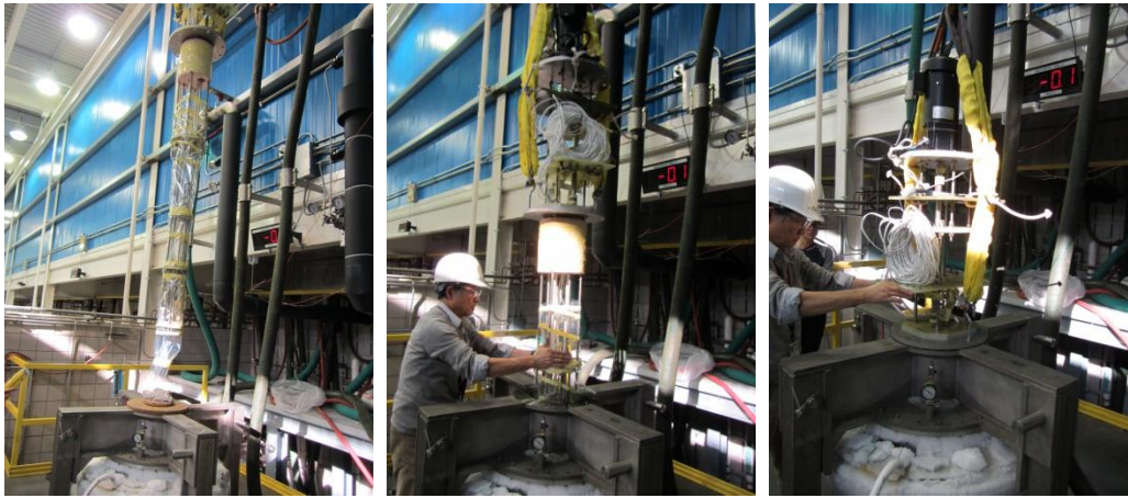
Figure 6.14 – Lowering of the probe into the cryostat.
