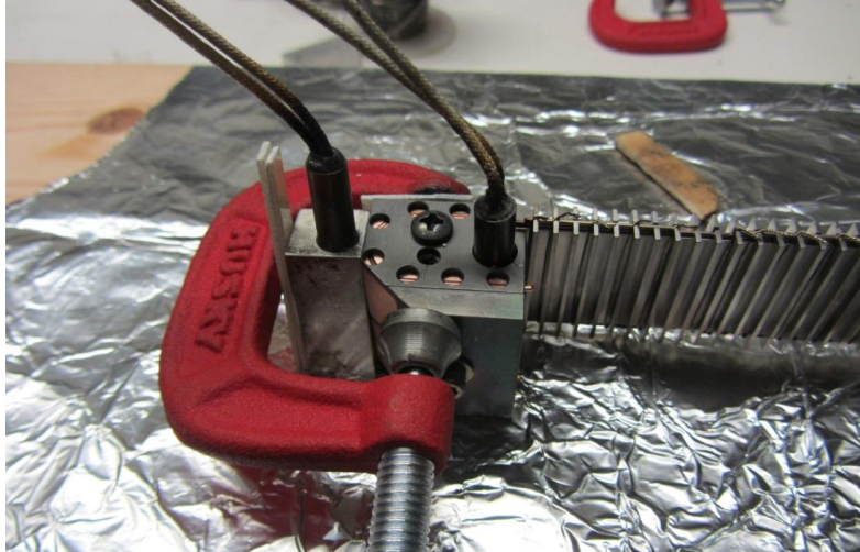
Figure 6.4 – Setup for soldering samples to current terminals.
