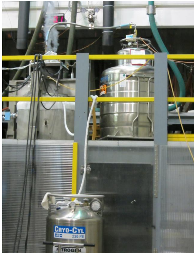
Figure 6.13 – Cryostat being filled with liquid nitrogen and liquid helium.
