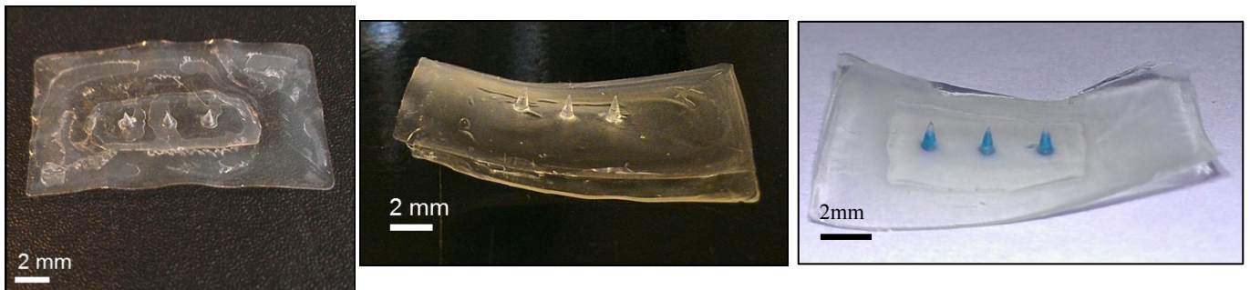
Figure 37. Progression of three needle devices with process development. Initial devices displayed poor lamination between layers (left). As the lamination process was improved, the appearance of the devices did as well (middle) and it was even demonstrated that a third component could be included between the needles and backing in the needle divot that formed during drying of these larger structures. This could allow further development into a device with multiple programmable release kinetics.
