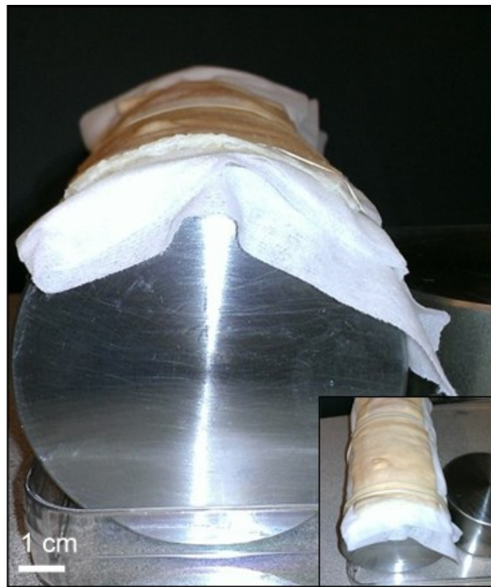
Figure 11. Curved porcine skin release model. The setup for evaluating release of a model drug into cadaver porcine skin consisted of the porcine skin sample placed over wet paper towels to maintain hydration. This sample was formed around a cylindrical stainless steel rod with 4.5cm radius of curvature, closely resembling a human forearm.
