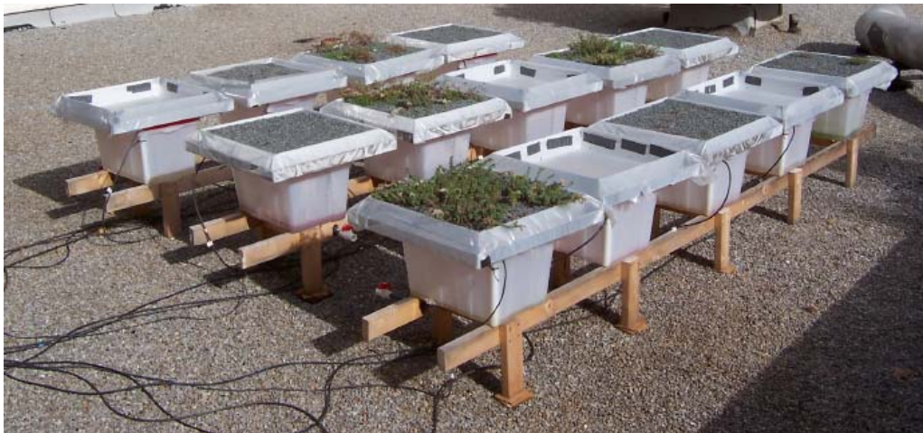
Figure 2.3 Experimental design of UGA modular green roof system
