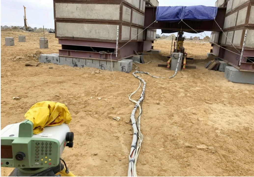
Figure 4-2 Digital-level instrument. Courtesy of Fugro Kazakhstan
