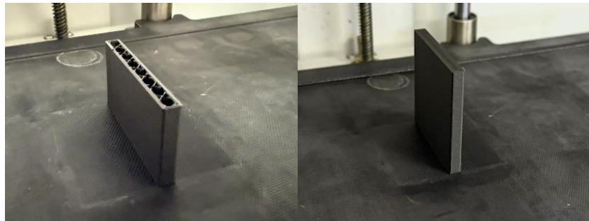
Fig. 7. Sample printed in the longitudinal infill orientation mid print and after completion.
