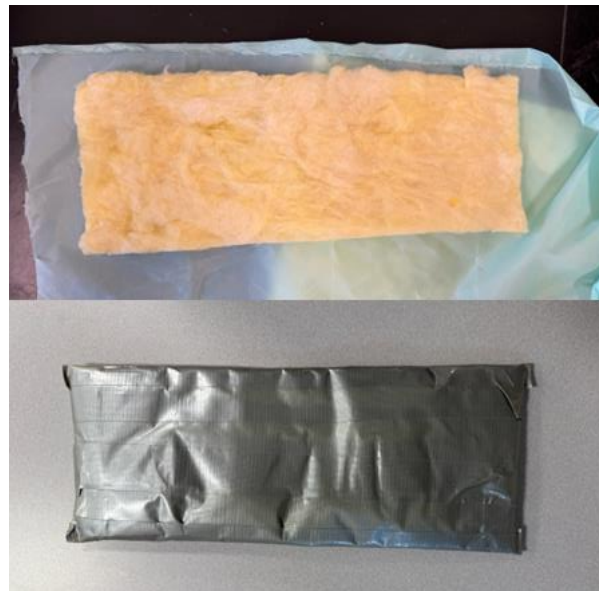
Fig. 15. Fiber glass sheet (Top). Insulation wrapped in duct tape and fabric sleeve (Bottom).
