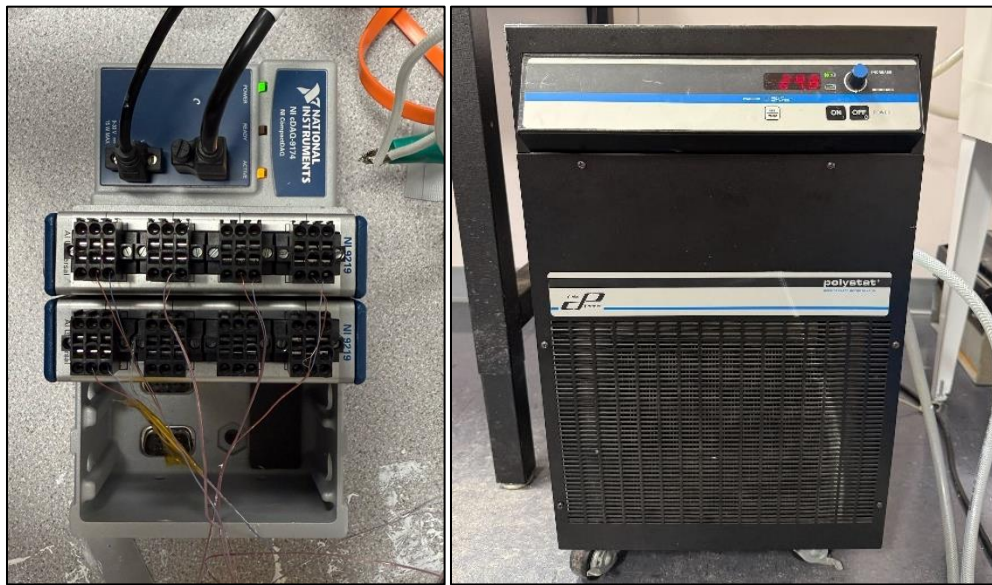
Fig. 18. National Instruments DAQ system (L) and Cole Palmer recirculating chiller (R).
