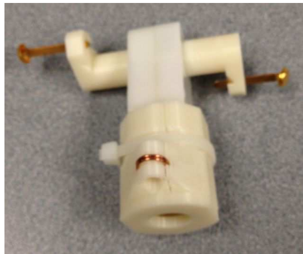
Fig. 4.2. PaperBots Robotics Kit Motor, modified from Solarbotics GM3, with added housing and hubs. (Photo by author)
