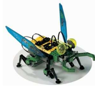
Fig. 1.5. Digital image of a LEGO Mindstorms RCX project. (Image available from www.microworlds.com )
