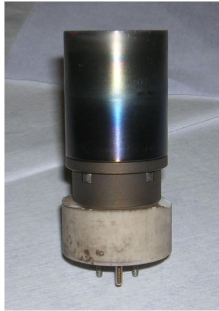
Figure 4-4: Plasma source base and anode before cleaning.
