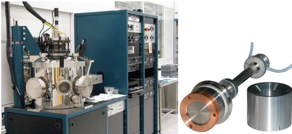
Figure 3-1: The 6-target sputtering system at CNS and a magnetron sputtering gun [2, 7]
