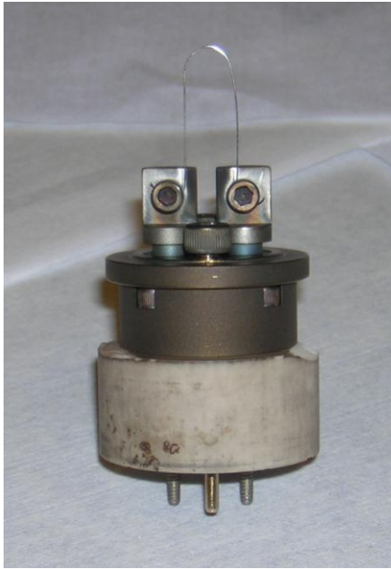
Figure 4-3: Plasma source base and cathode before cleaning.
