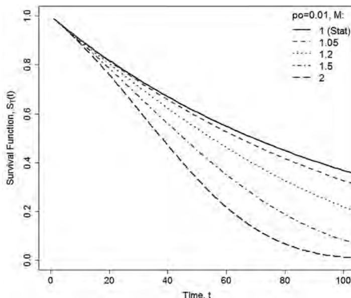
**Figure 2.** Survival function,  $S_T(t)$  (reliability) corresponding to flood series which arise from a nonstationary (EXP1) model with  $p_o = 0.01$ ; lines represent trends parameterized by a range of decadal magnification factors ( $M = 1, 1.05, 1.2, 1.5, \text{ and } 2$ ).
