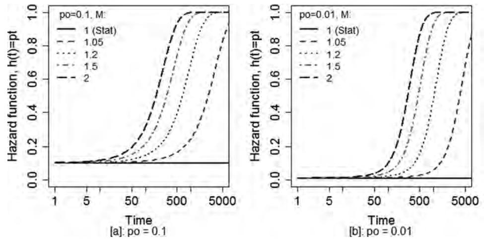
**Figure 1.** Hazard rate function  $h(t) = p_t$  corresponding to flood series which arise from a nonstationary EXP1 model; lines represent trends parameterized by a range of decadal magnification factors ( $M = 1, 1.05, 1.2, 1.5,$  and  $2$ ) for two possible event sizes: (a)  $p_o = 0.1$  and (b)  $p_o = 0.01$ . Note the log scale for the x axis (time).
