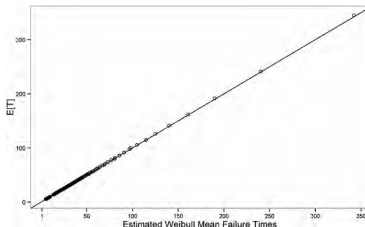
**Figure 9.** Comparison of exact values of average return period  $E[T]$  from (equation (6)) with regression estimates from a fitted Weibull-2 model in (24), (25), and (26). The data range represents a reasonable range of parameters from LN2 distributed flood flows ( $M = 1 - 2$ ;  $C_x = 0.25 - 1.5$ ;  $p_o = 0.001, 0.01, \text{ and } 0.1$ ).
