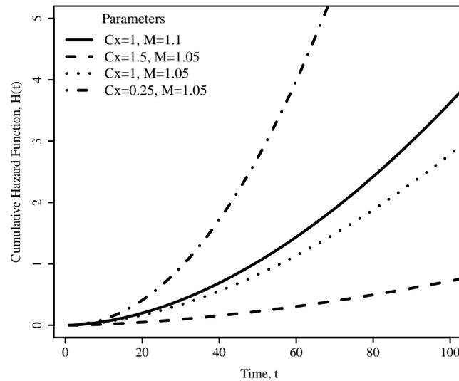
**Figure 8.** Cumulative hazard function  $H(t)$  for simulated time to failure data corresponding to flood series arising from a nonstationary LN2 model; traces illustrate parameter subsets for the  $p_o = 0.01$  event corresponding to a range of values of coefficient of variation  $C_x$  and Magnification factor,  $M$ .
