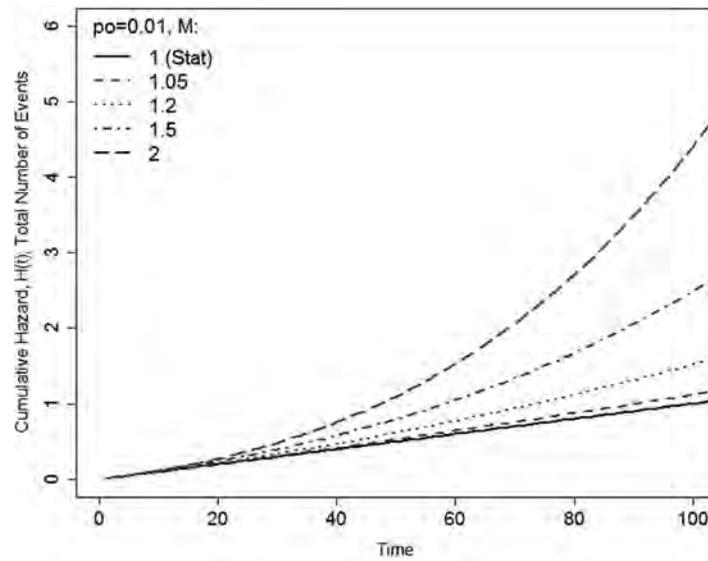
**Figure 3.** Cumulative hazard function,  $H(t)$  corresponding to PDS flood series which arise from a nonstationary EXP1 distribution with  $p_o = 0.01$ ; lines represent trends parameterized for a range of magnification factors ( $M = 1, 1.05, 1.2, 1.5,$  and  $2$ ).
