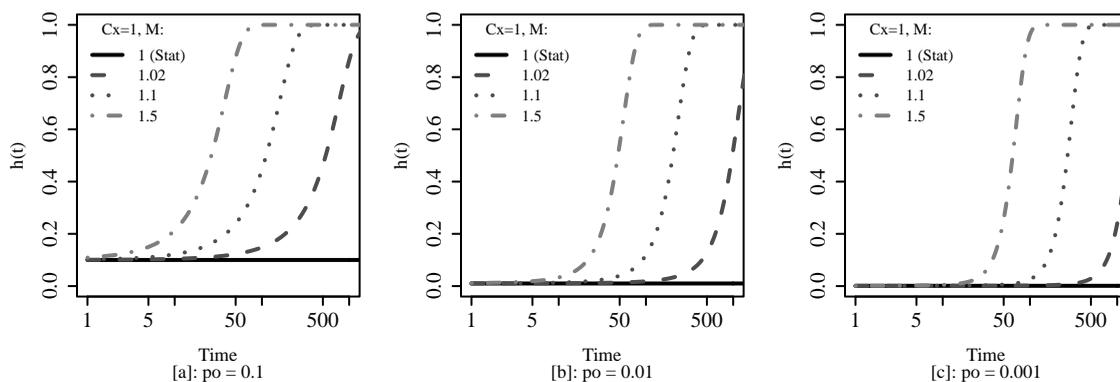
**Figure 5.** Hazard function  $h(t) = p_t$  corresponding to nonstationary LN2 flood series with  $C_x = 1$ ; dotted and dashed lines represent increasing trends ( $M = 1.01, 1.05, 1.1, \text{ and } 1.5$ ) from stationary ( $M = 1$  solid black) illustrating evolution in each plot for different sized events: (a)  $p_o = 0.1$ , (b)  $p_o = 0.01$ , and (c)  $p_o = 0.001$ .
