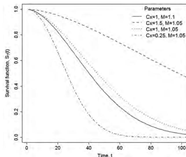
**Figure 7.** Survival function of simulated time to failure data corresponding to a nonstationary LN2 flood series; traces illustrate parameter subsets for the  $p_o = 0.01$  event corresponding to a range of values of coefficient of variation  $C_x$  and Magnification factor,  $M$ .
