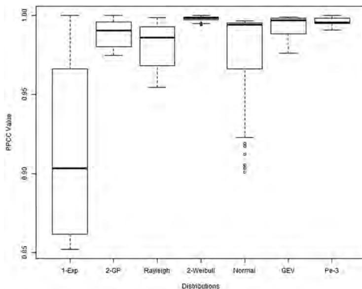
**Figure 6.** Boxplots of PPCC values that illustrate goodness of fit of simulated failure time data corresponding to nonstationary LN2 flood series for a range of parameters ( $M$ : 1–2;  $C_x = 0.25$ –1.5;  $p_o = 0.001, 0.01, \text{ and } 0.1$ ) to a range of models including the Exponential (1-EXP), Generalized Pareto (2-GP), Rayleigh, 2-Weibull, Normal, Generalized Extreme Value (GEV), and Pearson Type III (Pe-3) distributions.
