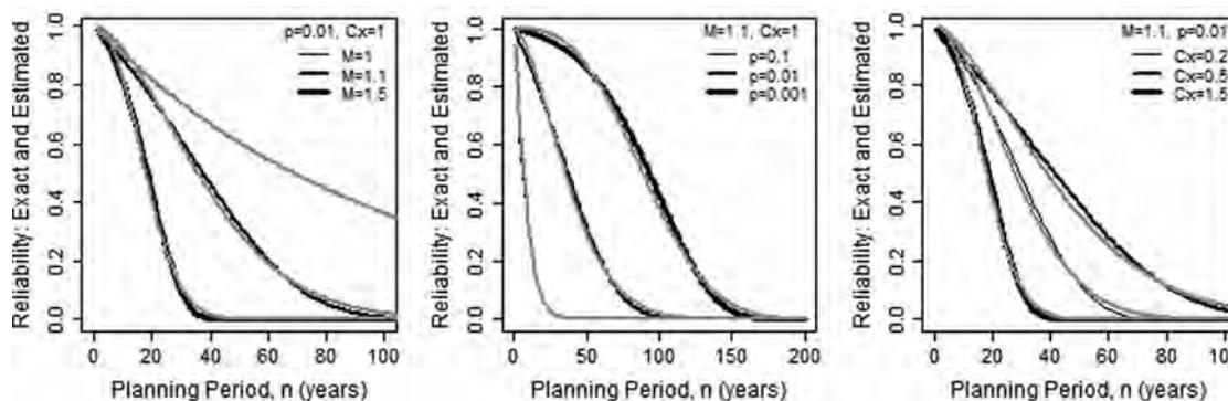
**Figure 10.** Comparison of reliability values corresponding to nonstationary LN2 flood series using exact simulation results (black lines) with Weibull-2 regression model estimates (grey lines) for a range of experimental values: (a) trends,  $M = 1$  (stationary), 1.1, and 1.5; (b)  $p_o = 0.1, 0.01$ , and 0.001; (c)  $C_x = 0.2, 0.5$ , and 1.5.
