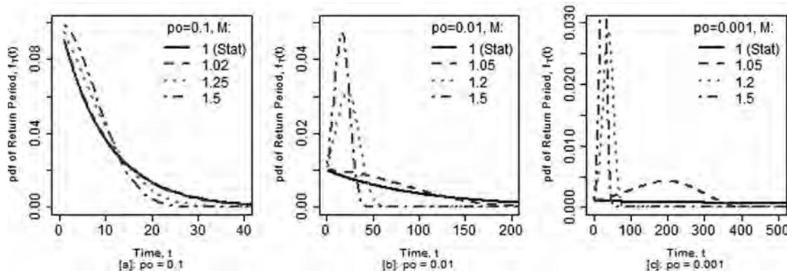
**Figure 4.** The pdf of the distribution of the return period  $T$  corresponding to a nonstationary EXP1 model; each figure shows a range of possible trend values considering a range of magnification factors ( $M = 1, 1.02, 1.25,$  and  $1.5$ ) and plots are per event size: (a)  $p_o = 0.1$ , (b)  $p_o = 0.01$ , and (c)  $p_o = 0.001$ .
