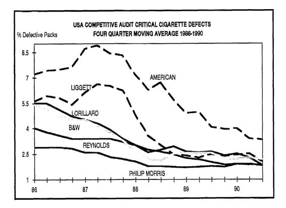
The emphasis will be to reduce the cigarette defect level by 50% with particular focus on functional defects (void ends, torn rod, open seam, etc.) which are a major cause of consumer complaints.
