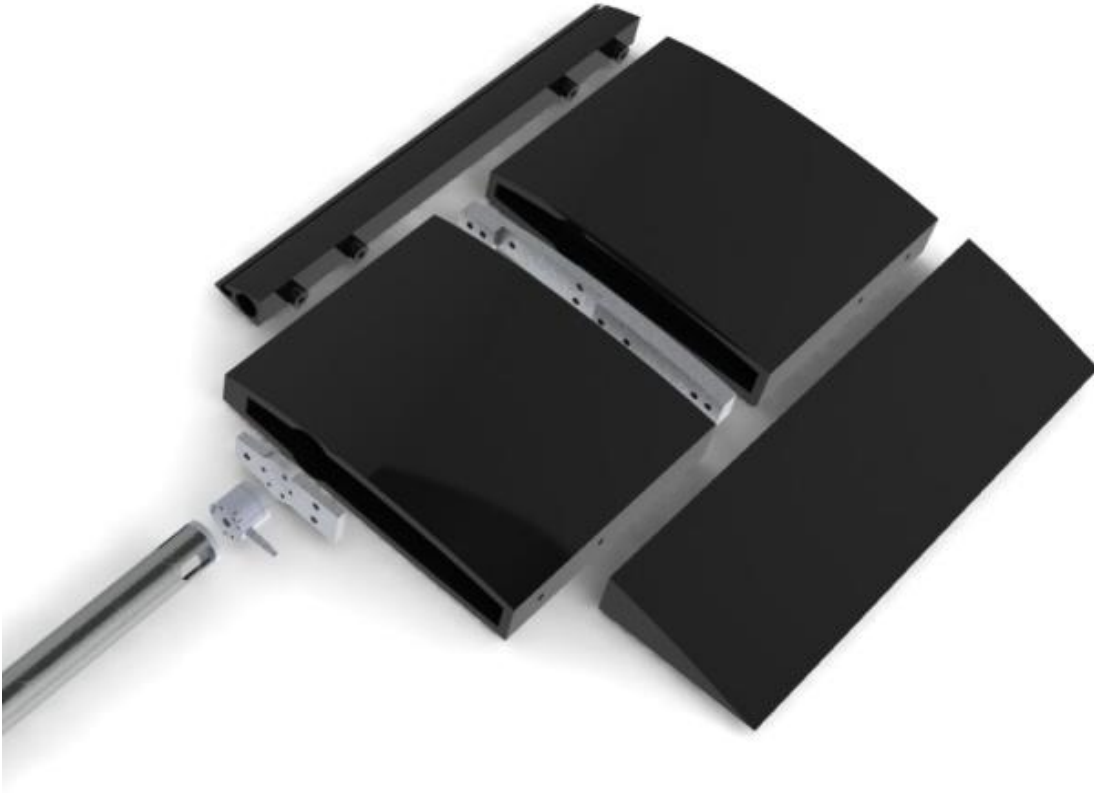
Figure 10 - Airfoil model exploded view including all for airfoil elements, centerline plate, sensor mounting plate, the Nano25 force sensor and Sting assembly
