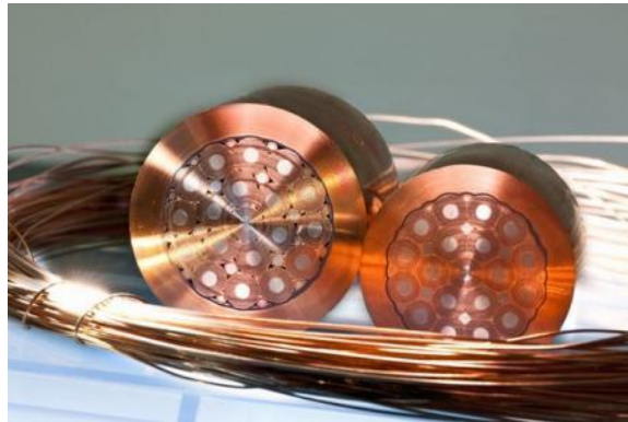
Figure 5 - Nb 3 Sn Billet Example [6]
