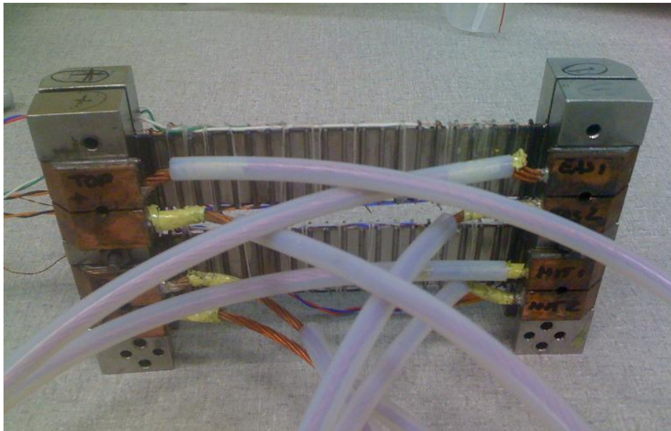
Figure 26 - Sample Holders Mounted on Vertical Arms
