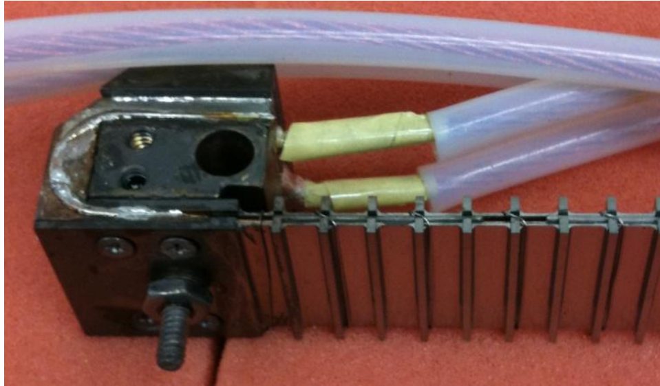
Figure 15 - Sample Holder with Current Terminators and Leads
