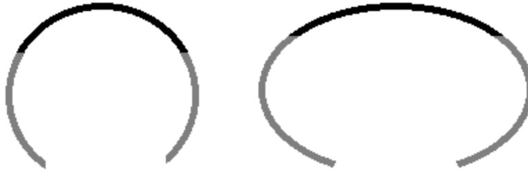
Figure 44 - Bending Schematic. Left: Desirable deformation; Right: Undesirable deformation (not to scale)
