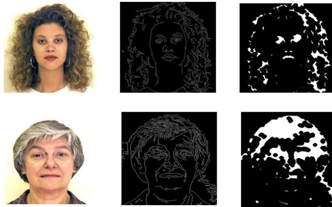
Figure 4.20: Comparison of results using the Canny edge detector with custom threshold values (Low Threshold = .08; High Threshold = 0.2)
