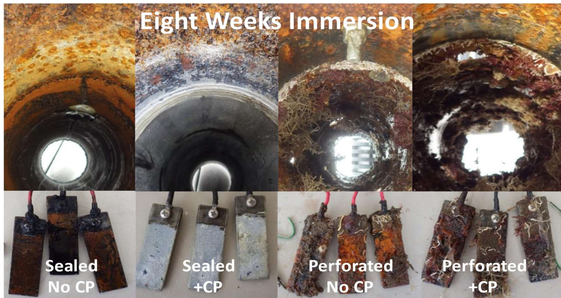
Figure 25 Images of biofouling within perforated vs unperforated pipes. Reproduced with permission
