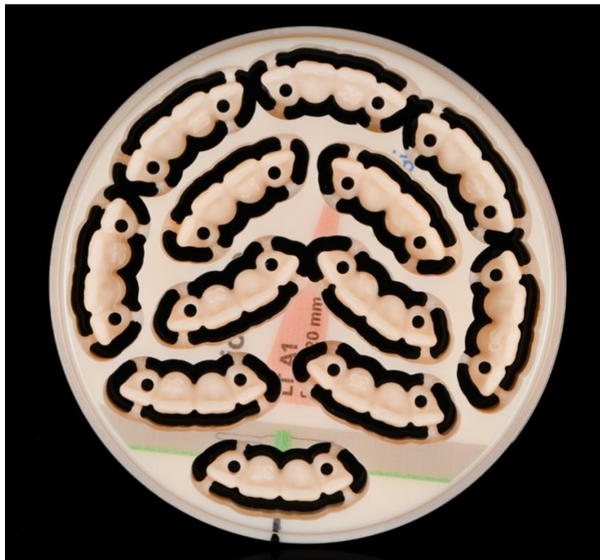
Figure.7: PMMA Prototypes after milling
