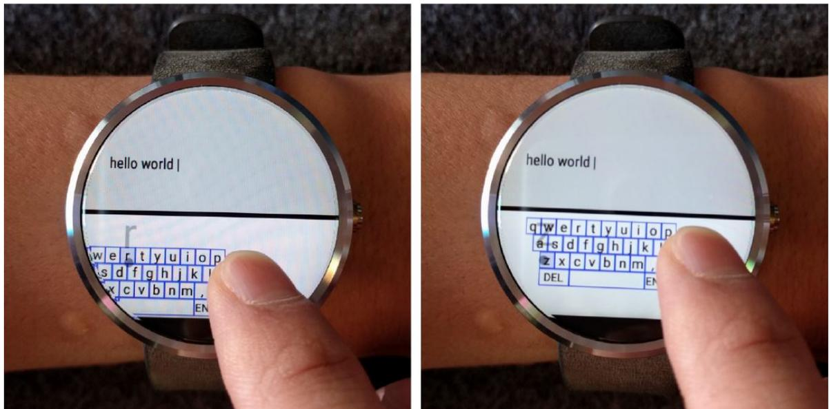
**Figure 4:** DriftBoard prototype in action on a smartwatch with a round display (Motorola Moto 360). Left, the fixed cursor is on top of "r". Right, the location of the fixed cursor remains the same, but it acquires "z" as the result of keyboard movement. Note that in the DriftBoard concept, the size of the movable keyboard is not necessarily the same as the device' frame size. Note also that DriftBoard is applicable to more shapes than just a rectangle.
