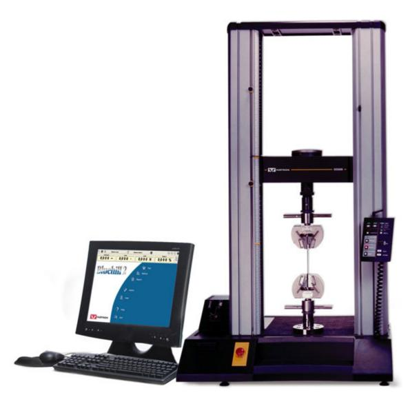
Figure 13: Universal testing machine.
