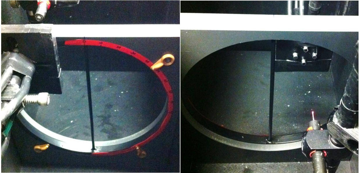
Figure 2.4 Pictures of the circular gantry used to hold the black Delrin rod. The circular gantry allows for angular movement in the x - y plane, while the frame that holds the gantry allows for angular movement in the x - z plane.
