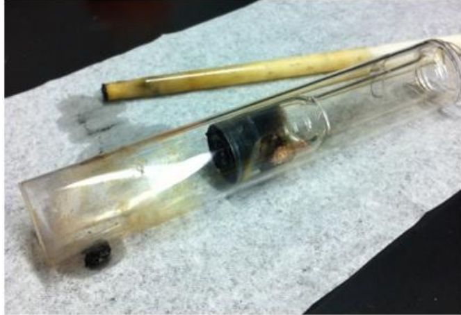
Figure 27: Carbon buildup (black residue) on ICP injector after sampling
