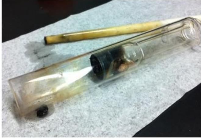
**Figure 27: Carbon buildup (black residue) on ICP injector after sampling**
