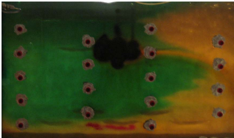
Figure 28. Aquifer Cell #2: 0.75 Pore Volumes of Dyed Tracer Introduction
