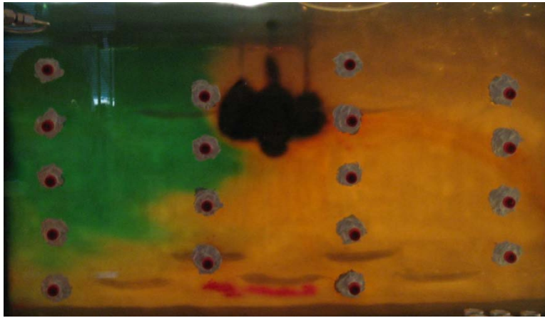
Figure 26. Aquifer Cell #2: 0.35 Pore Volumes of Dyed Tracer Introduction
