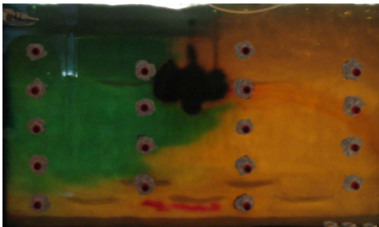
Figure 27. Aquifer Cell #2: 0.5 Pore Volumes of Dyed Tracer Introduction
