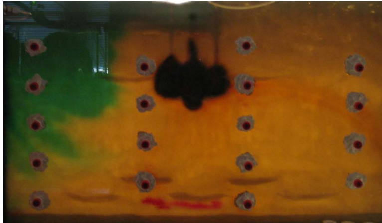
Figure 25. Aquifer Cell #2: 0.2 Pore Volumes of Dyed Tracer Introduction
