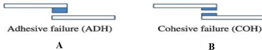
Figure (12): Representation of failure modes characteristics of adhesive joints submitted to shearing (A) Adhesion failure, detachment material from surface. (B) Cohesive failure, debonds material from inside
