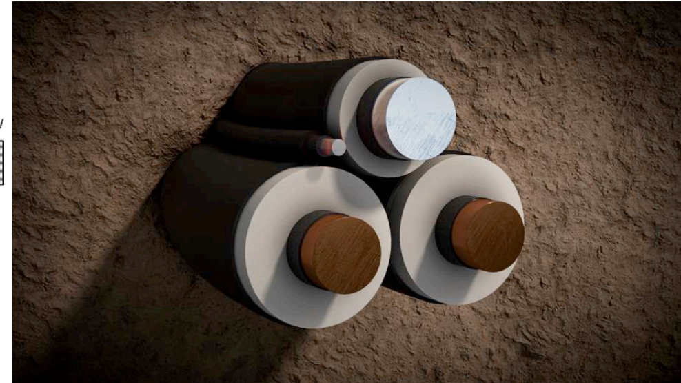
Bi-pole cable with metallic return
