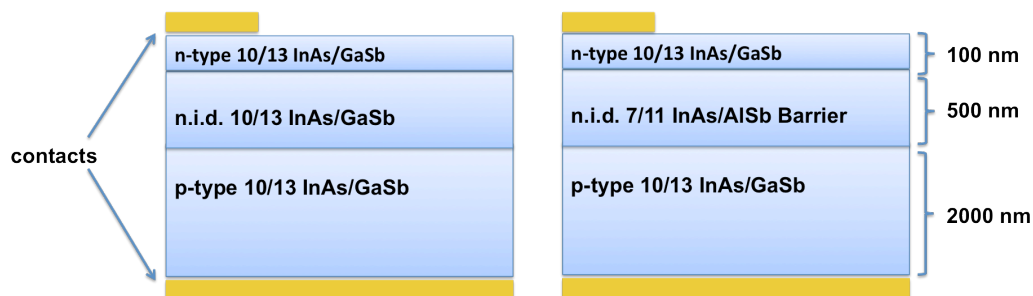
Figure 6-7: Device stack for the pin (left) and barrier (right) diodes.
