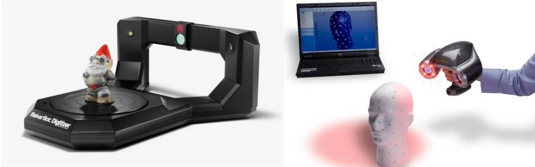
Figure 5: On the left, a first-generation portable 3D scanner, the MakerBot Digitizer. On the right, a second generation portable scanner, the ZScanner. Images sourced from 3ders.org and engadget.com , respectively.
