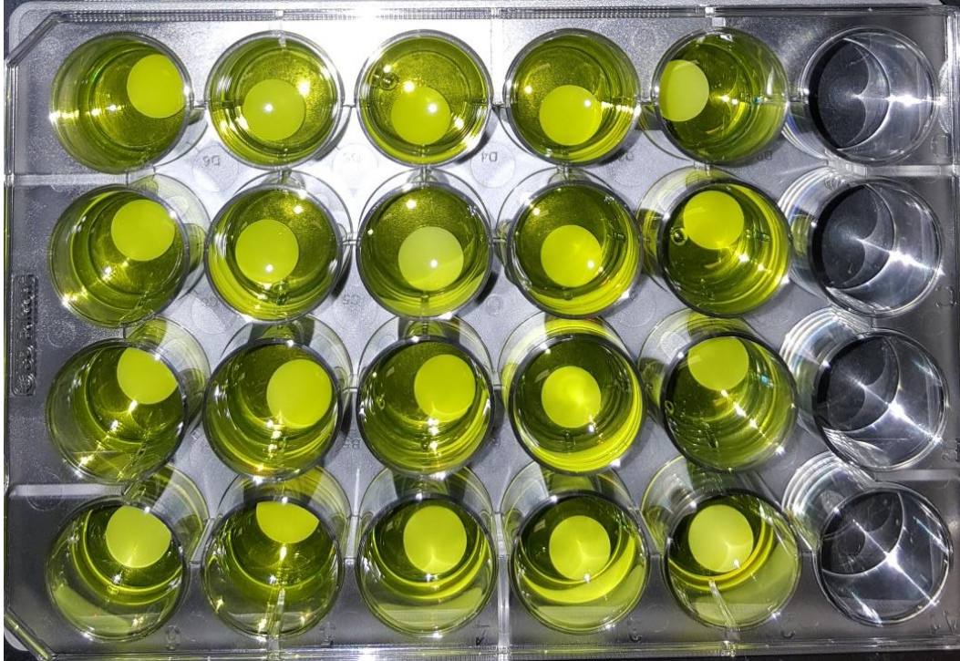
Figure 20: Gels from condition four were treated exactly the same as gels from condition three, but they were exposed to blue light for the first hour of the glycerol bath.
