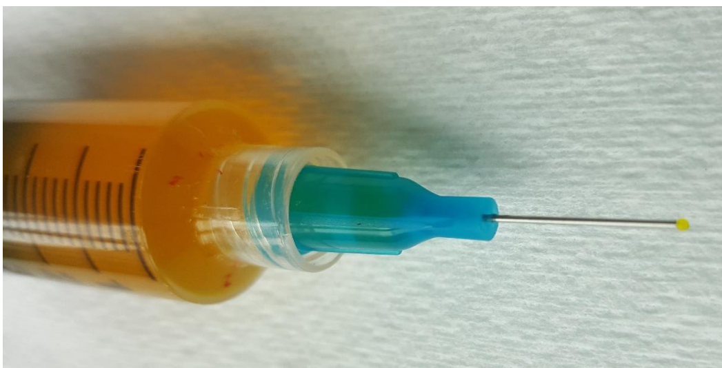
Figure 16: A drop of riboflavin-infused ink is extruded from a probe needle with an inner diameter of 300\mu\text{m} . For reference, a human body cell can have a diameter between 10 and 100\mu\text{m} 30 .
