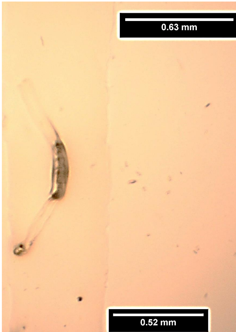
Figure 27: A microscopic photo of a single printed filament showing the variation in its width in one short segment and the presence of impurities.
