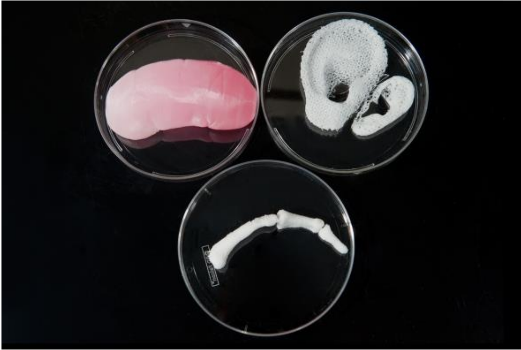
Figure 42: Rudimentary printed tissue replacements. The kidney organoid, top left, was printed with kidney cell inks. Source: Ledford, 2015
