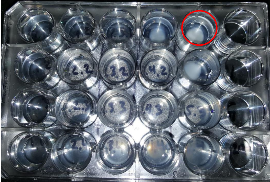
Figure 23: Gels from condition seven are almost invisible because they contain no riboflavin, which provides the yellow coloration in other samples, and no glycerol, so the silk does not crosslink. Only the one highlighted biopsy survived to be tested.
