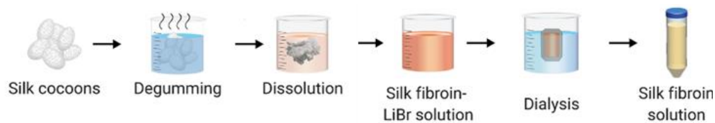
Figure 20: Degumming process of silk fibroin. Silk cocoons are boiled to remove sericin, dissolved in lithium bromide solution, which is then dialyzed to remove lithium bromide leaving SF in pure water. Figure adapted with permission from Guidetti et al 2022.
