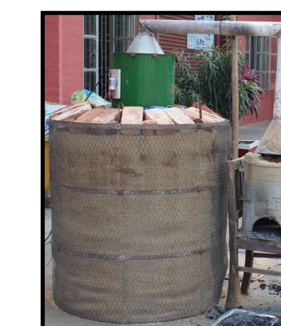
BAU-STR dryer developed at Bangladesh Agricultural University in association with PHLIL.
