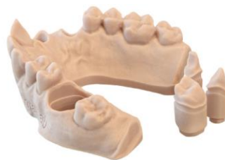
Figure 5: 3D printed alveolar cast with removable dies, illustrating the precision of digital manufacturing in dental prosthesis creation.
