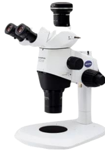
Figure 6: Olympus microscope used for precision measurement at 5X magnification during evaluation.
