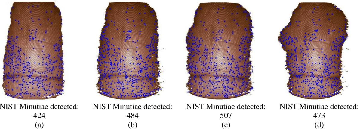
Figure 8: (a) shows the detected minutiae on the unrolled images of the original, and (b-d) shows the minutiae on unrolled images of the deformed models.
