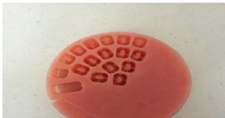
Figure 3. Avadent CAD/CAM pack during milling process
