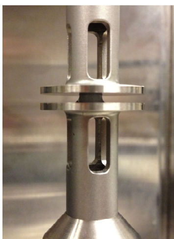
Figure 7 Loaded sample with platens at nominal gap of \leq 2mm.
