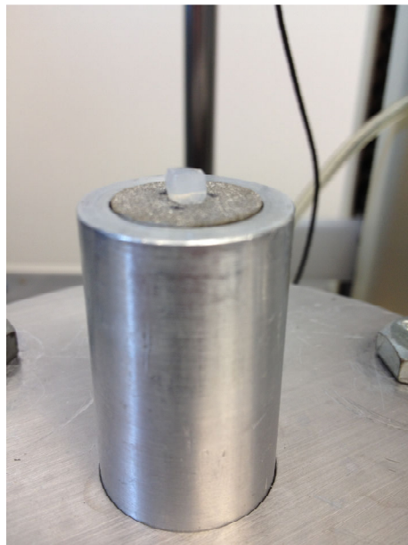
Figure 5 Ultra-fine porous steel filtering disc used for drainage of water from the samples during equilibrium.
