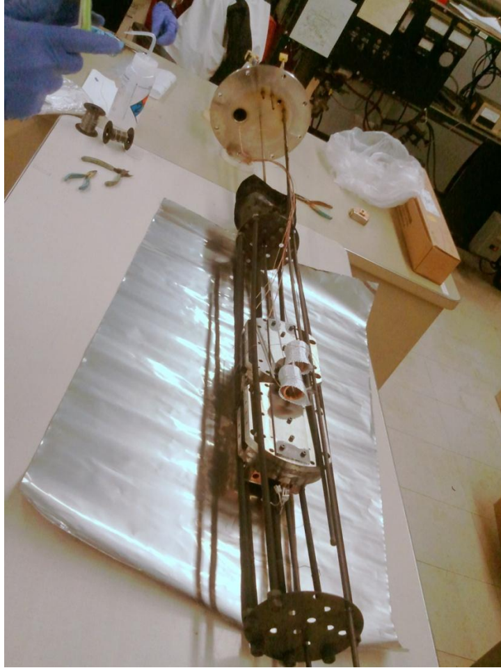
Fig. 3.13 Two transverse experimental assemblies ready to go into the oven for heat treatment. Notice the assembly is up-side down to fit better in the oven holder.
