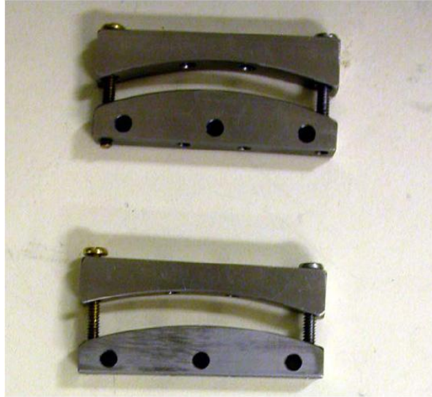
Fig. 1.16 Fixed pure bending strain sample holders [9].
