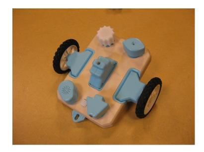
Figure 3. The KIWI Robot with its modular sensors, motors and light output
